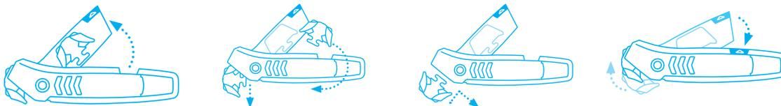
Swing open the **blade magazine**. The fitted blade head will automatically disengage.
